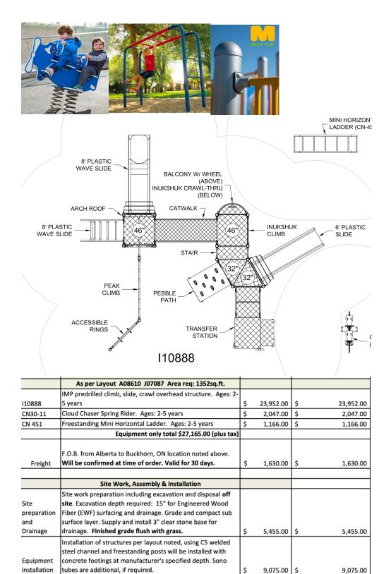
Supply and Install 12" compacted depth of Engineered Wood Fiber (CSA accessibility compliant) over geo-textile filter cloth
